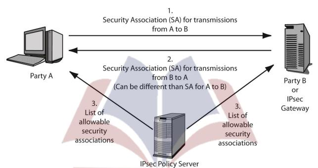
When a device receives a packet via the IPSec protocol, it is the SA that tells the device what to do with the packet. So if device B receives a packet from device C via IPSec, device B will look to the corresponding SA to tell it how to decrypt the packet, how to properly authenticate the source of the packet, which key to use, and how to reply to the message if necessary.
