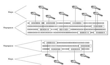
keys that would be possible. That would not be a very large keyspace, and certainly it would not take an attacker very long to find the correct key that was used. A large keyspace allows for more possible keys. Today, we are commonly using key sizes of 128, 256, 512, or even 1,024 bits and larger. So a key size of 512
