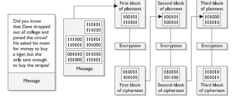
your friend. He has to have the same block cipher and key, and those 10 ciphertext blocks go back through the algorithm in the reverse sequence and end up in your plaintext message.
