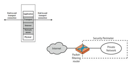
(a) Packet-filtering router
