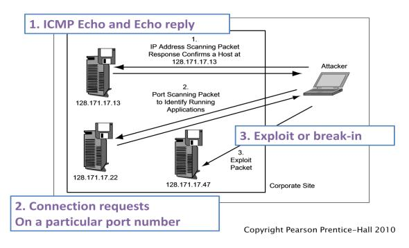
**The exploit:** The specific attack method that the attacker uses to break into the computer is called the attacker's exploit. The act of implementing the exploit is called exploiting the host
