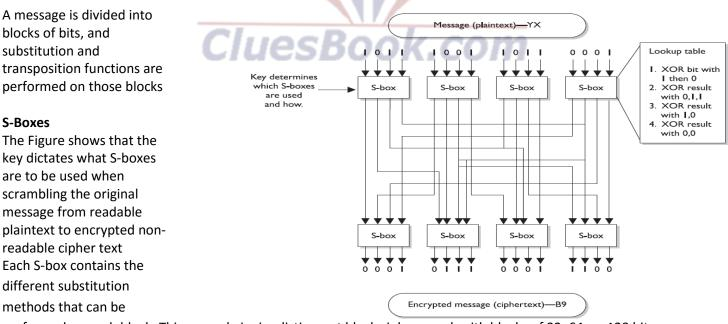
performed on each block. This example is simplistic most block ciphers work with blocks of 32, 64, or 128 bits in size, and many more S-boxes are usually involved
