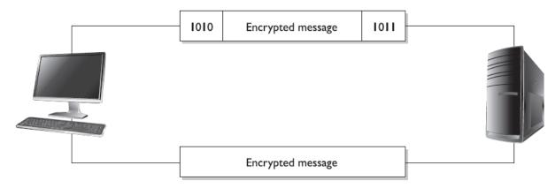
Link encryption happens at lower layers and encrypts headers and trailers of the packet.
