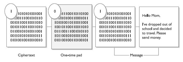
The receiver must have the same one-time pad to decrypt the message, by reversing the process. The receiver takes the first bit of the encrypted message and XORs it with the first bit of the pad. This results in the plaintext value.
